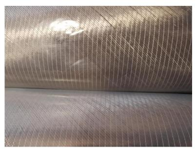
Non-crimp multiaxial technical textiles or fabrics made from multiple layers of unidirectional placed and stitch bonded FILAVA™ fibers permits to obtain higher tensile strength and flexural properties in the reinforced composite materials.
