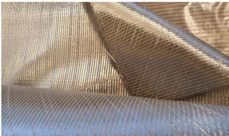
processes where a great mechanical strength combined with visual quality finishes are required, like hand lay-up, injection or infusion molding and RTM composite processes. Due to the genuine and tailored sizings applied on the fibers during the stretching process, non-crimped multi-axial fabrics are ideally
